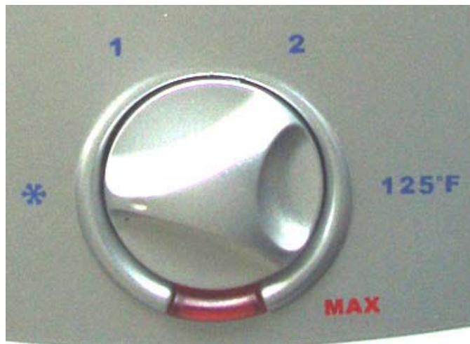
Temperature adjusting knob in "Freeze Protection" position
